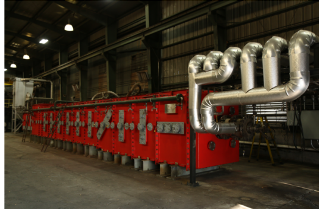
L1500 furnace (1.1 m x 1.1 m cross section, 13.1 m in length)
