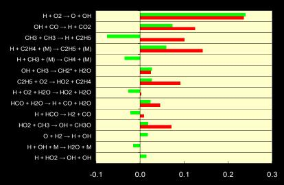
laminar flame speed in a stoichiometric atmospheric  $C_2H_6$ -air mixture
