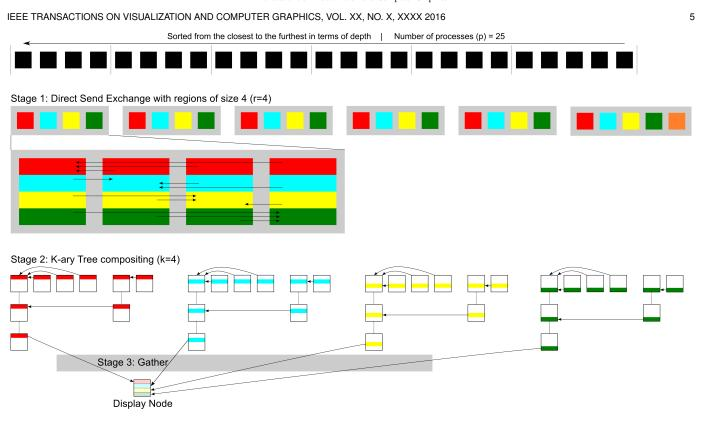
Fig. 2: The three stages of the compositing algorithm with r=4, k=4, and the number of nodes p=25. Red, blue, yellow and green represent the first, second, third and fourth quarters of the image.
