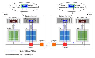
Fig. 1: Inter-node GPU communication with and without GPU Direct RDMA.
