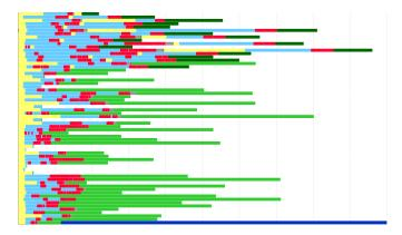
Fig. 5: Profile for 64 nodes for 2048x2048 (64MB) image on Edison at NERSC with r=16, k=8. Red: compositing, green: sending, light blue: receiving, dark blue: receiving on the display process. Total time: 0.012s.
