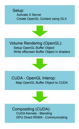
Fig. 4: Workflow for GPU rendering.
